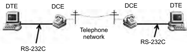
Fig. 9.78 Data flow between computer terminals and modems
